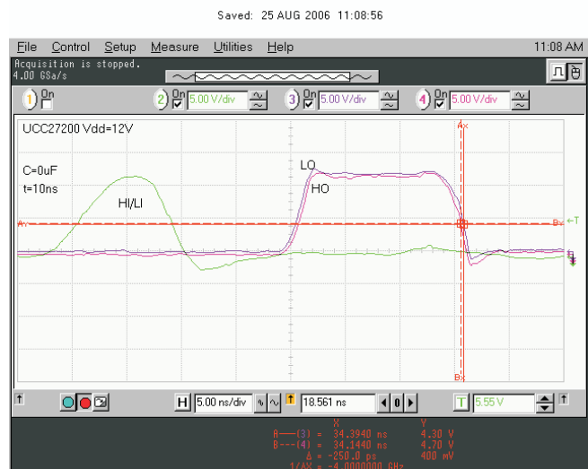
Figure 34. 10-ns Input Pulse Delay Matching
