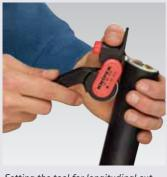
Setting the tool for longitudinal cut
