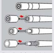
Dismantling of a Coax-cable in three steps
