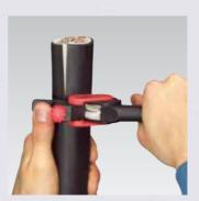
Turning the tool for circular cut
