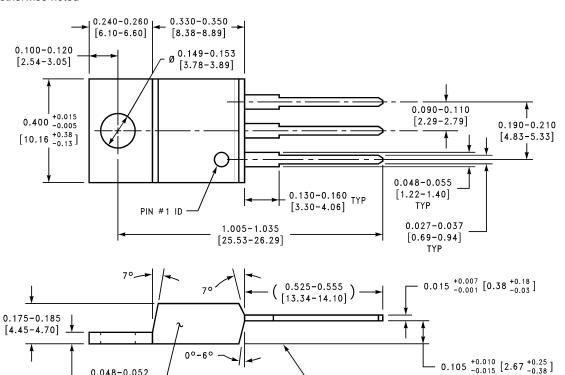
TO-220 3-Lead Molded Package Order Number LM2930T-5.0 or LM2930T-8.0 **NS Package Number T03B**
