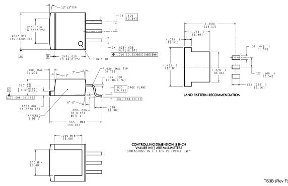
TO-263 3-Lead Plastic Surface Mount Package Order Number LM2930S-5.0 or LM2930S-8.0 **NS Package Number TS3B**
