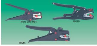
A range of automatic wire strippers to cover cable sizes  $0.25 \text{mm}^2$  to  $6.00 \text{mm}^2$ . They all operate using a unique system of self adjusting multiple blades which slice cleanly through the insulation but then form around the conductors to give a clean cut without causing any damage.
