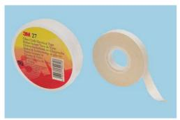
Scotch® 27 glass cloth electrical tape is a woven glass cloth tape designed to operate in applications requiring high mechanical strength and resistance to high temperatures. The glass cloth is specially treated and prepared to providecorrosion free protection. The glass will not shrink, rot or burn and has a high tensile strength. The adhesive is a rubber pressure-sensitive thermosetting system. The tape is designed for continuous use at class "B" (130°C) temperature.
