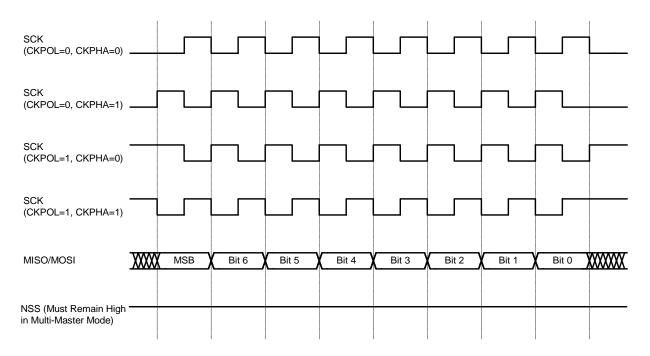
Figure 20.5. Master Mode Data/Clock Timing
