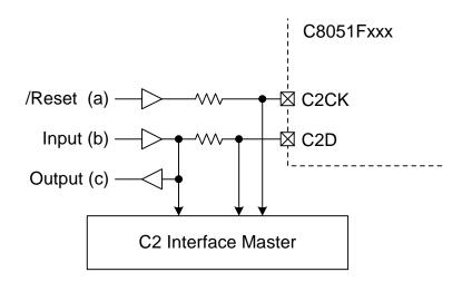
Figure 23.1. Typical C2 Pin Sharing
