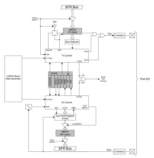
Figure 18.1. UARTO Block Diagram
