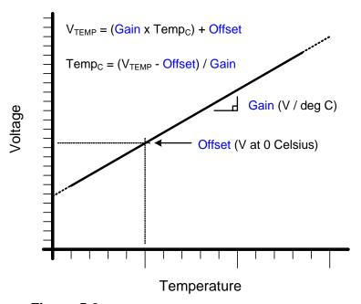
Figure 5.2. Temperature Sensor Transfer Function
