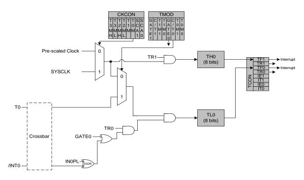
Figure 21.3. T0 Mode 3 Block Diagram
