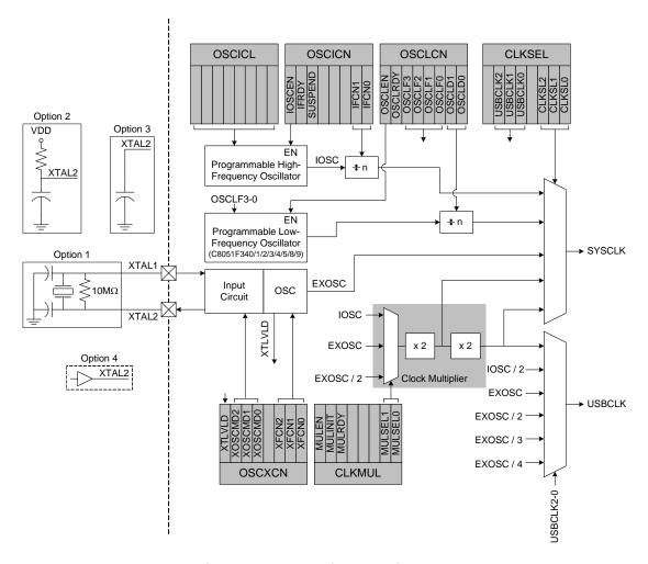
Figure 14.1. Oscillator Diagram
