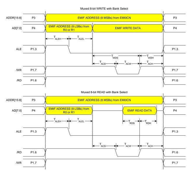
Figure 13.10. Multiplexed 8-bit MOVX with Bank Select Timing
