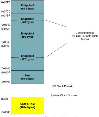
Figure 16.3. USB FIFO Allocation
