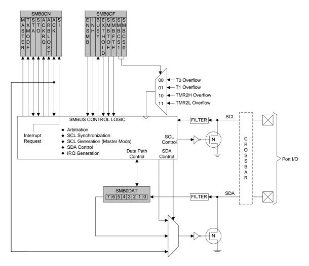
Figure 17.1. SMBus Block Diagram
