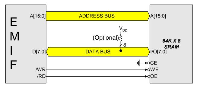
Figure 13.3. Non-multiplexed Configuration Example
