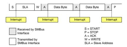
Figure 17.5. Typical Master Transmitter Sequence
