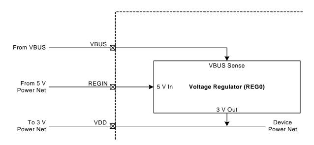
Figure 8.2. REG0 Configuration: USB Self-Powered
