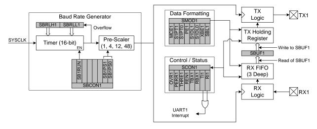
Figure 19.1. UART1 Block Diagram
