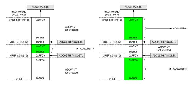
Figure 5.9. ADC Window Compare Example: Left-Justified Differential Data
