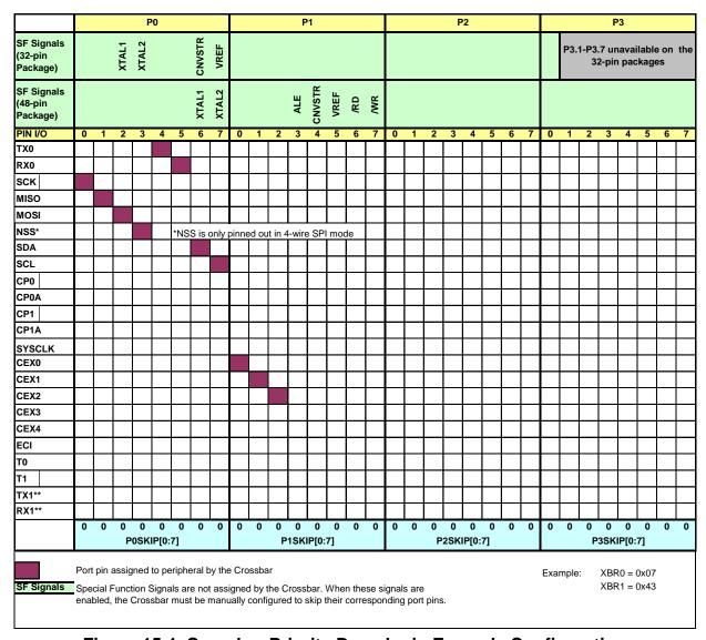
Figure 15.4. Crossbar Priority Decoder in Example Configuration (No Pins Skipped)
