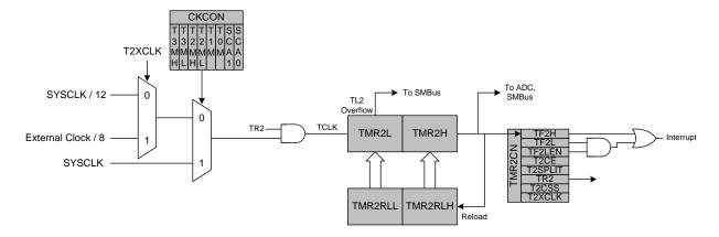
Figure 21.4. Timer 2 16-Bit Mode Block Diagram
