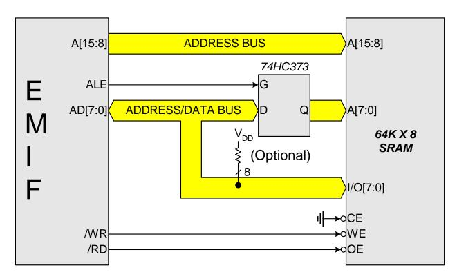
Figure 13.2. Multiplexed Configuration Example
