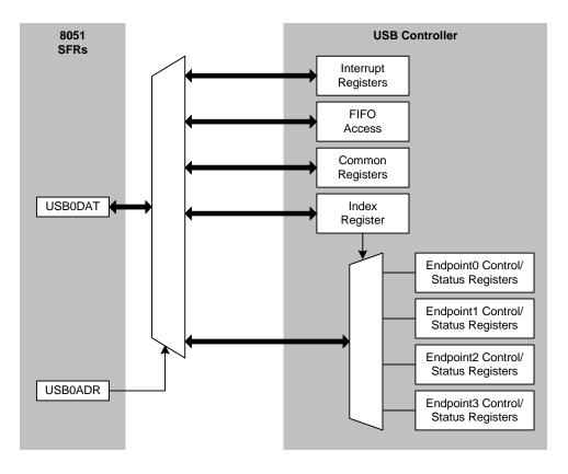
Figure 16.2. USB0 Register Access Scheme
