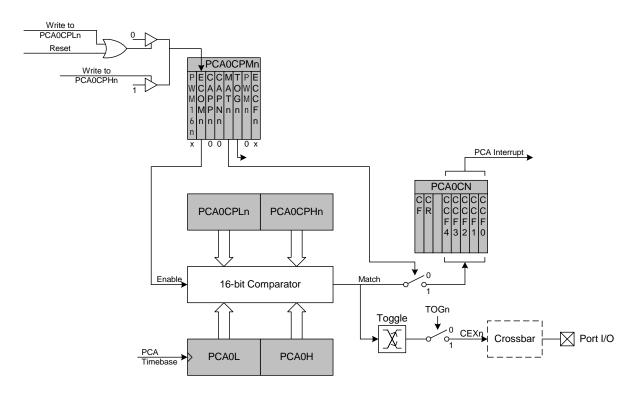
Figure 22.6. PCA High Speed Output Mode Diagram
