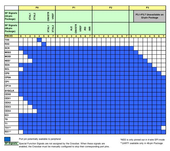
Figure 15.3. Peripheral Availability on Port I/O Pins
