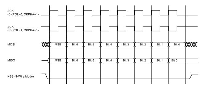
Figure 20.7. Slave Mode Data/Clock Timing (CKPHA = 1)
