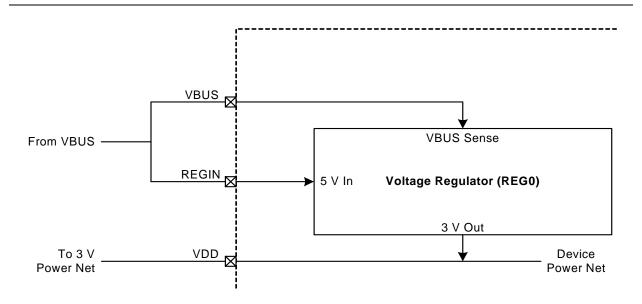
Figure 8.1. REG0 Configuration: USB Bus-Powered
