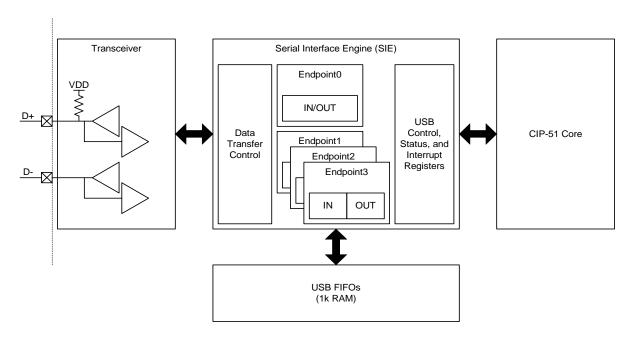
Figure 16.1. USB0 Block Diagram
