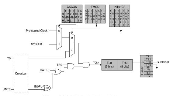
Figure 21.1. T0 Mode 0 Block Diagram
