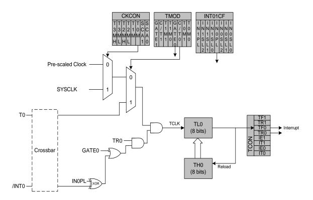
Figure 21.2. T0 Mode 2 Block Diagram
