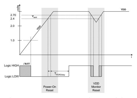
Figure 11.2. Power-On and V<sub>DD</sub> Monitor Reset Timing
