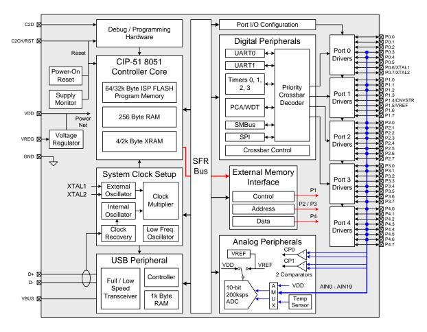
Figure 1.1. C8051F340/1/4/5 Block Diagram
