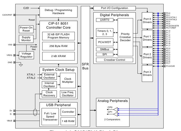
Figure 1.4. C8051F349 Block Diagram
