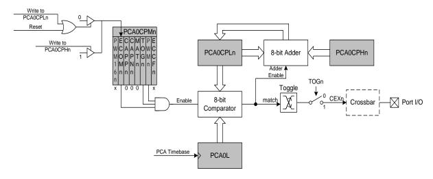
Figure 22.7. PCA Frequency Output Mode
