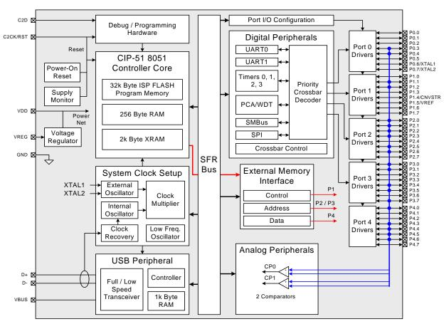
Figure 1.3. C8051F348 Block Diagram
