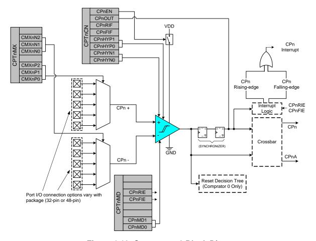
Figure 1.13. Comparator Block Diagram
