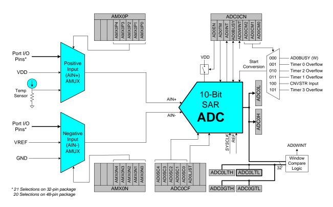
Figure 5.1. ADC0 Functional Block Diagram
