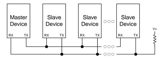
Figure 19.6. UART Multi-Processor Mode Interconnect Diagram
