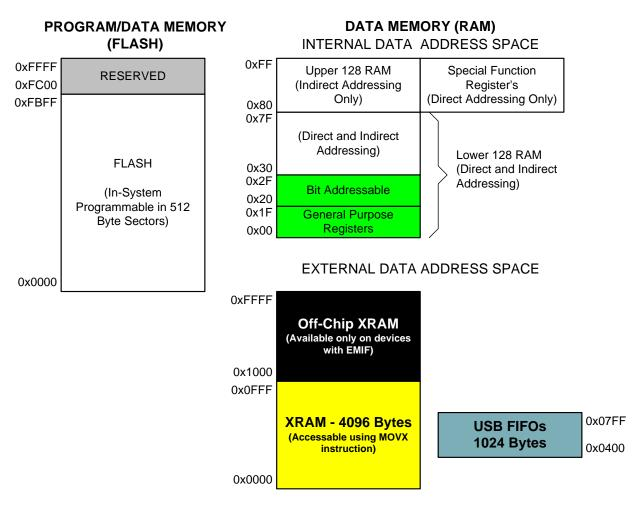
Figure 9.2. On-Chip Memory Map for 64 kB Devices (C8051F340/2/4/6)
