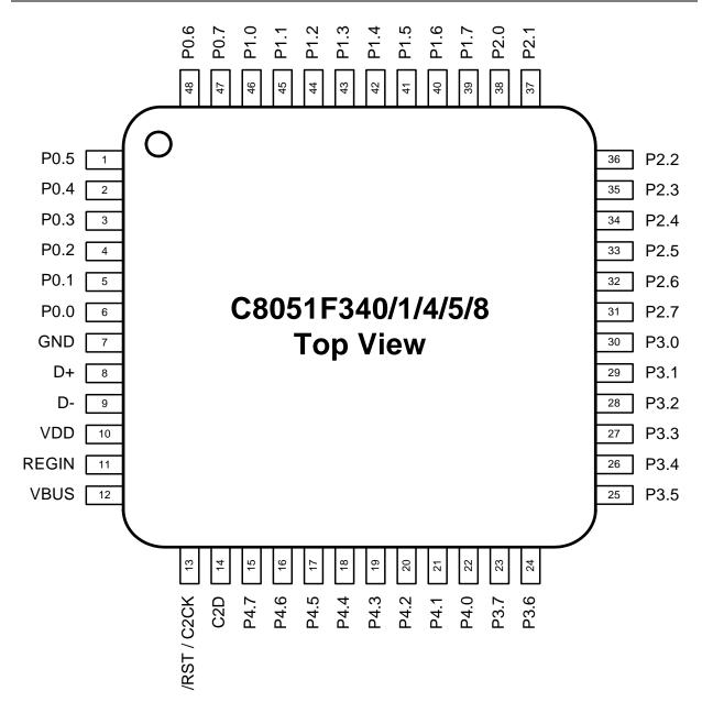
Figure 4.1. TQFP-48 Pinout Diagram (Top View)
