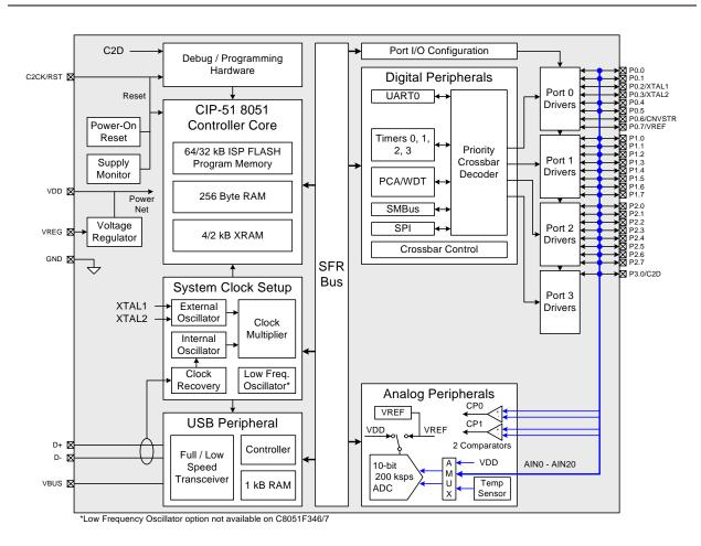
Figure 1.2. C8051F342/3/6/7 Block Diagram
