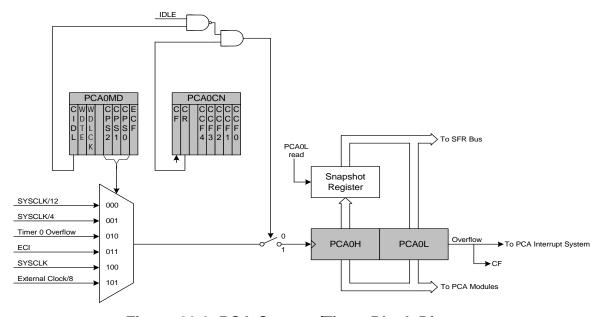
Figure 22.2. PCA Counter/Timer Block Diagram
