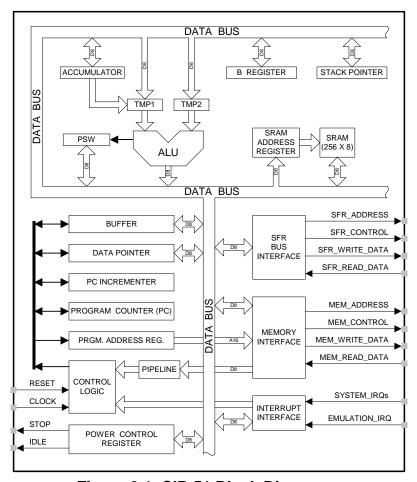
Figure 9.1. CIP-51 Block Diagram
