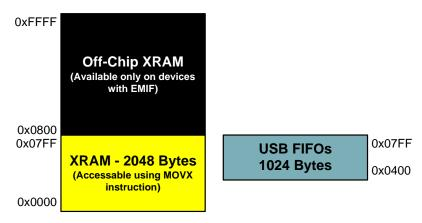
Figure 1.7. On-Chip Memory Map for 32 kB Devices (C8051F341/3/5/7/8/9)
