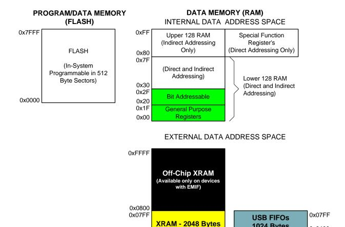
Figure 9.3. On-Chip Memory Map for 32 kB Devices (C8051F341/3/5/7/8/9)
