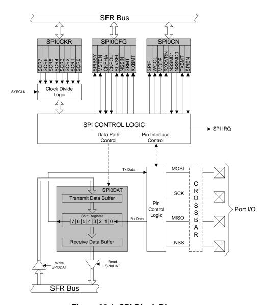
Figure 20.1. SPI Block Diagram
