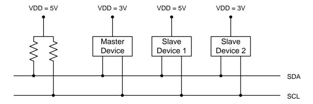
Figure 17.2. Typical SMBus Configuration
