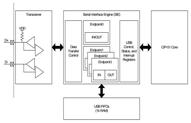
Figure 1.8. USB Block Diagram
