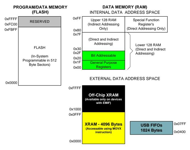
Figure 1.6. On-Chip Memory Map for 64kB Devices (C8051F340/2/4/6)
