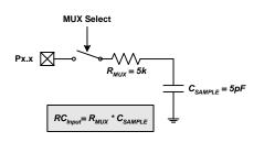
Figure 5.5. ADC0 Equivalent Input Circuits
