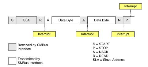
Figure 17.8. Typical Slave Transmitter Sequence
