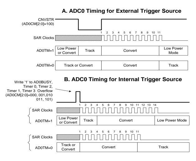
Figure 5.4. 10-Bit ADC Track and Conversion Example Timing
