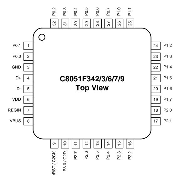
Figure 4.3. LQFP-32 Pinout Diagram (Top View)
