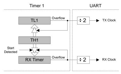
Figure 18.2. UARTO Baud Rate Logic
