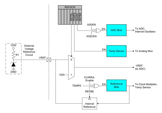
Figure 6.1. Voltage Reference Functional Block Diagram
