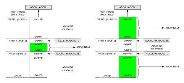
Figure 5.8. ADC Window Compare Example: Right-Justified Differential Data
