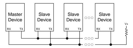
Figure 18.6. UART Multi-Processor Mode Interconnect Diagram
