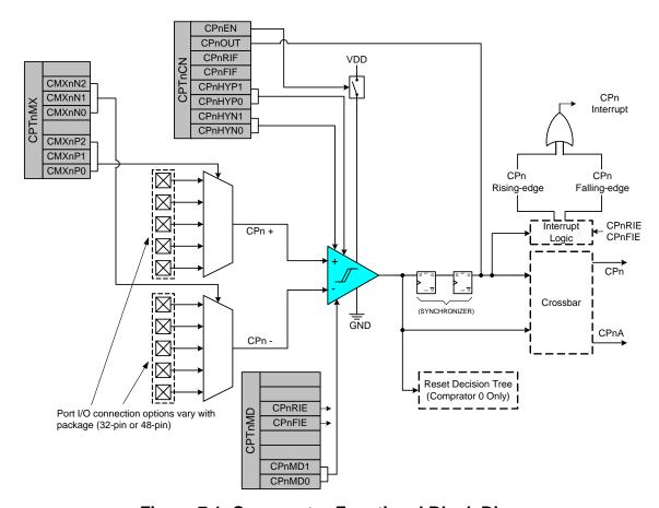
Figure 7.1. Comparator Functional Block Diagram
