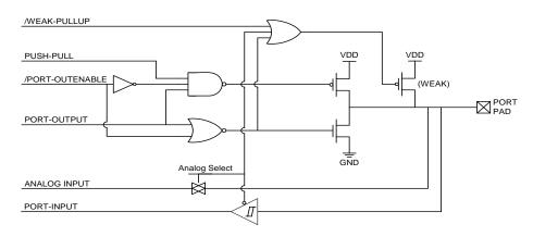
Figure 15.2. Port I/O Cell Block Diagram
