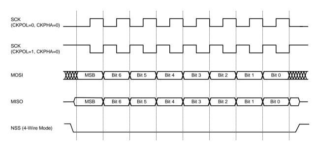
Figure 20.6. Slave Mode Data/Clock Timing (CKPHA = 0)
