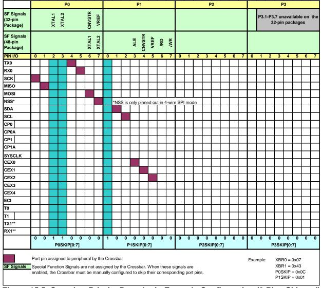
Figure 15.5. Crossbar Priority Decoder in Example Configuration (3 Pins Skipped)
