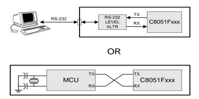
Figure 18.3. UART Interconnect Diagram
