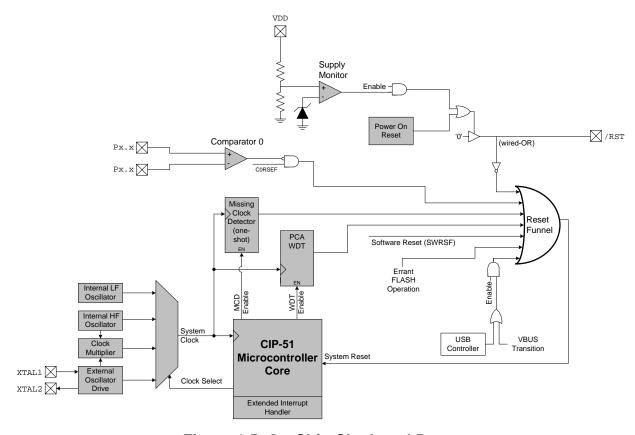
Figure 1.5. On-Chip Clock and Reset
