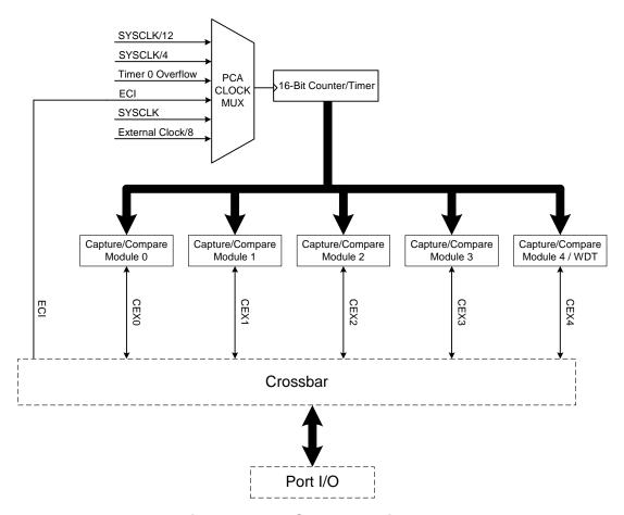
Figure 22.1. PCA Block Diagram
