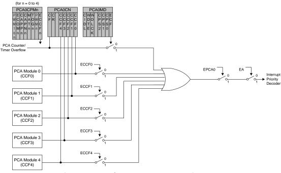
Figure 22.3. PCA Interrupt Block Diagram
