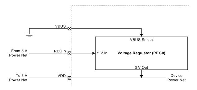
Figure 8.4. REG0 Configuration: No USB Connection
