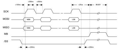
TTL Synchronous serial communication.
