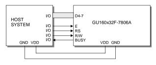
The data bus width can be selected for 4-bit operation, using data lines D4-D7. Within this mode, two writes are required to send one data byte. The high nibble (bits 4-7) should be sent first, followed by the low nibble (bits 0-3). The busy state is not triggered between nibbles. It is important that the status is NOT read within 40us of sending the command to set either 4 or 8 bit mode.
