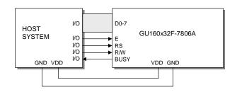
The busy state can be monitored on D7 when reading the DDRAM address (RS line low). The busy state can also be monitored directly from CN1 pin 3 if link J6 is set to 2&3.
