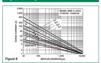
NOTE: If pulse ratings are exceeded, a shift of  $V_{N(DC)}$  (at specified current) of more than +/-10% could result. This type of shift, which normally results in a decrease of  $V_{N(DC)}$  may result in the device not meeting the original published specifications, but it does not prevent the device from continuing to function, and to provide ample protection.
