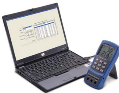
Figure 1: Automate the recording of continuous readings when you hook the U1731A/32A to a PC
