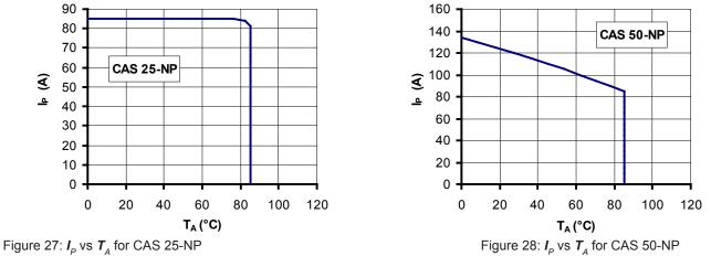
The maximum continuous DC primary current plot shows the boundary of the area for which all the following conditions are true:
