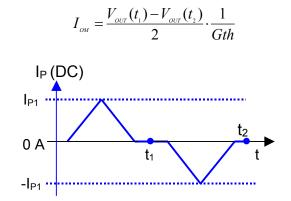
Figure 30: Current cycle used to measure magnetic and electrical offset (transducer supplied)
