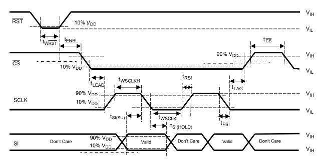
Figure 7. Input Timing Switching Characteristics
