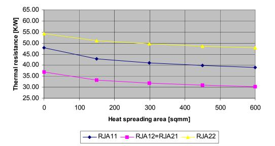
Figure 20. Steady State Thermal Resistance in Dependence on Heat Spreading Area; 1s JEDEC Thermal Test Board with Spreading Areas
