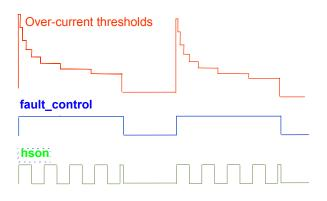
In steady state, the wire harness will be protected by OCLO2 current level by default. Three other DC over-current levels are available: OCLO1 or OCLO3 or OCLO4 based on the state of the OCLO[1,0] bits.
