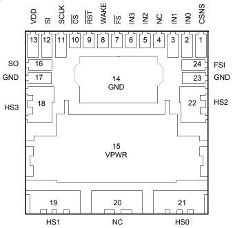
Figure 3. 10XS3435 Pin Connections
