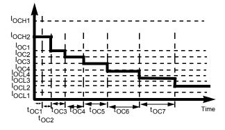
Figure 15. Over-current Profile with OCHI Bit Set to '1'
