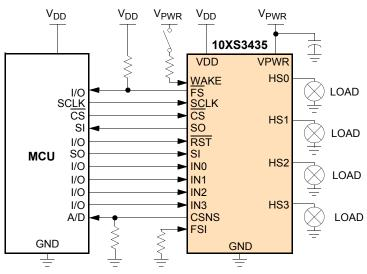
Figure 1. 10XS3435 Simplified Application Diagram
