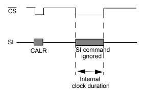
In case of negative  $\overline{\text{CS}}$  pulse is outside a predefined time range (from  $t_{\text{CSB}(\text{MIN})}$  to  $t_{\text{CSB}(\text{MAX})}$ ), the calibration event will be ignored and the internal clock will be unaltered or reset to default value ( $f_{\text{PWM}(0)}$ ) if this was not calibrated before.
