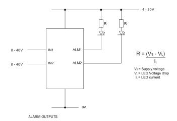
Applications that feature an alarm can be connected as above. ALM1 and ALM2 must not sink more than 10mA maximum each. If supply voltage varies, use an appropriate voltage regulator.
