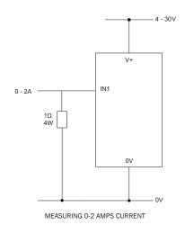
Use a 1  $\Omega$  resistor, with a 4W rating. Setup scaling in software: 0V = 0.00 and 2V = 2.00
