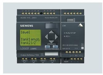
Using the AS-Interface connection for LOGO!, an intelligent slave can be integrated in the AS-Interface system. With the modular interface it becomes possible to integrate the different basic units in the system according to their functionality. Similarly, functionalities can be quickly and easily adapted to new requirements by exchanging the basic unit.
