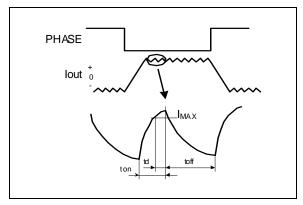
FIGURE 3-3: PWM Output Current Waveform
