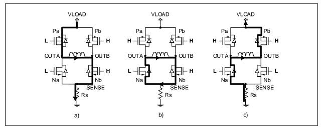
**FIGURE 3-1:** Power bridge control (PHASE = H / forward): (a) bridge ON, (b) source OFF, and (c) all OFF / coasting (for PHASE = L / reverse: invert A and B in drawings)
