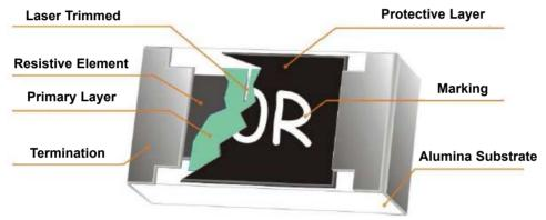
Figure 1. Construction of a Chip-R
