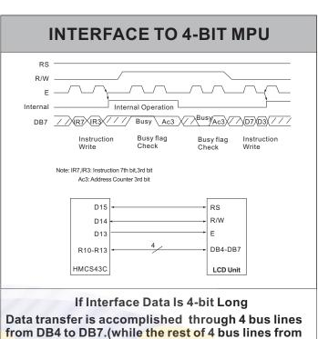
Data transfer is completed when 4-bits of data is transferred twice.(upper 4-bits of data, then lower
