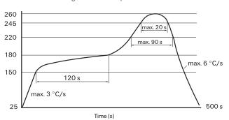
Infrared Soldering: temperature/ time profile (lead and housing peak temperature) Tape and reel for SMT version 480 relays per reel, 2400 relays per box
