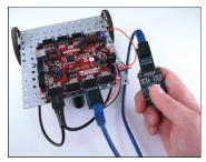
The Remote kit provides the components need to build a wired remote control robot. It combines the RSK and Cerebot 32MX4 with a joystick module and 10' control cable.
