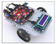
The Basic kit provides the components needed to build a simple autonomous robot. It combines the RSK and Cerebot 32MX4 with a push button module, a switch module and a character LCD module.
