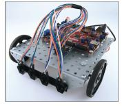
The Line Sensor kit provides the components needed to build a line following robot. It combines the RSK and Cerebot 32MX4 with the optical sensor module, optical sensors, and mounting bracket.
