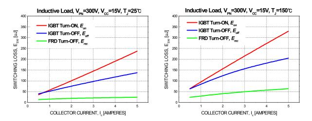
Figure 5. Switching Loss Characteristics
