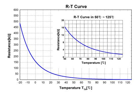
Figure. 6. R-T Curve of The Built-in Thermistor
