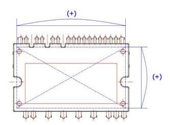
Figure 9. Flatness Measurement Position
