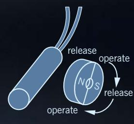
Multi-pole ring magnets can be used to achieve a larger number of operations per rotation
