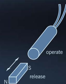
Both ends of the magnet work equally well
