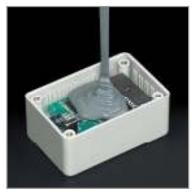
polyurethanes, epoxies, silicones and many other polymers, each system will have advantages as well as limitations. It is therefore, important to fully understand the chemical and physical properties of each system and carefully match these to the requirements of the component and manufacturing processes.
