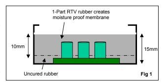
1-Part condensation cure (RTV) products should not be used where the depth of encapsulant is more than 10mm, see **Fig 1**, as it will cure to form a moisture proof membrane and prevent the cure in the bottom of the enclosure.
