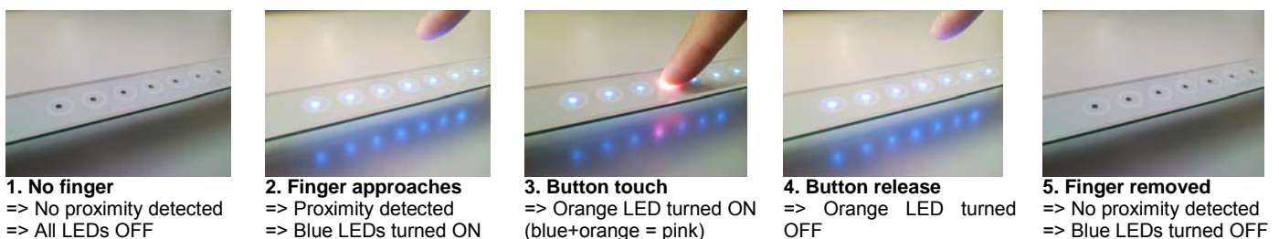
Figure 66 Touch+Proximity Module Operation
