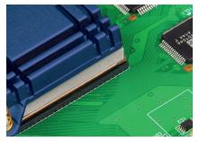
Gap Pad® VO Ultimate is a robust, highly compliant product that is ideal for both small and large gap designs. The fiberglass carrier on one side of the material allows ease of rework, excellent handling characteristics and puncture resistance. Additionally the fiberglass carrier has a slight inherent tack, minimizing any shifting during assembly.
