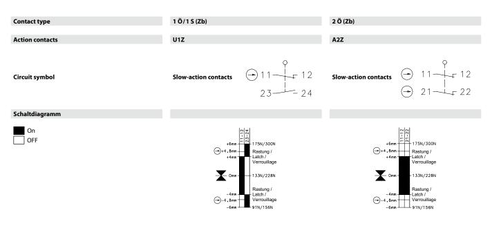
The pulling force data depend on the type of switch used. (SRM...175/SRM...300) Tolerances: Switching point +/- 0.5 mm, actuating force +/- 15 %
