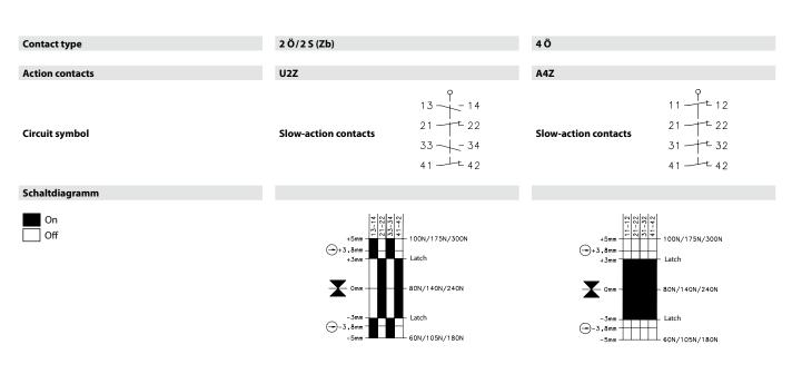
The pulling force data depend on the type of switch used. (SR...100/SR...175/SR...300) Tolerances: Switching point +/- 0.5 mm, actuating force +/- 15 %
