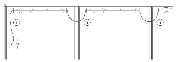
This illustration shows the LED 025 lamp in a daisy chain application. The lamps are conveniently connected via quick connection plugs — up to 10 lamps max. can be daisy-chained this way. The snap lock connectors ensure a stable electrical connection even if subjected to heavy vibration. The connection example shows a 230VAC application, using the following cables: connection cable with female connector, Art. No. 244356 (1); daisy chain extension cable with 2 connectors, Art. No. 244358 (2).
