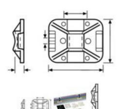
Each mount is designed to offer the maximum surface area, and in conjunction with the specially developed adhesive ensure that a very high pull-off force is achieved. The concave design of the mounts ensures that larger diameter cables and bundles are fully supported.
