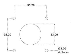
The body of the joystick is mounted from beneath the panel. The gaiter is passed through the panel cut-out and is held onto the front face of the panel by the mounting bezel. The square bezel has a gloss finish and is designed for use with No.4 x 3/8" pan head self tapping screws whereas the circular bezel has a matt finish and is designed for countersunk screws.
