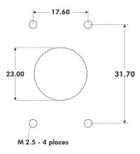
The joystick mounts from beneath the panel and the gaiter is trapped between the joystick and the panel. No bezel is necessary for this installation, since the panel acts as the bezel. The frame has M2.5 tapped holes and as such M2.5 machine screws are recommended for this mounting.
