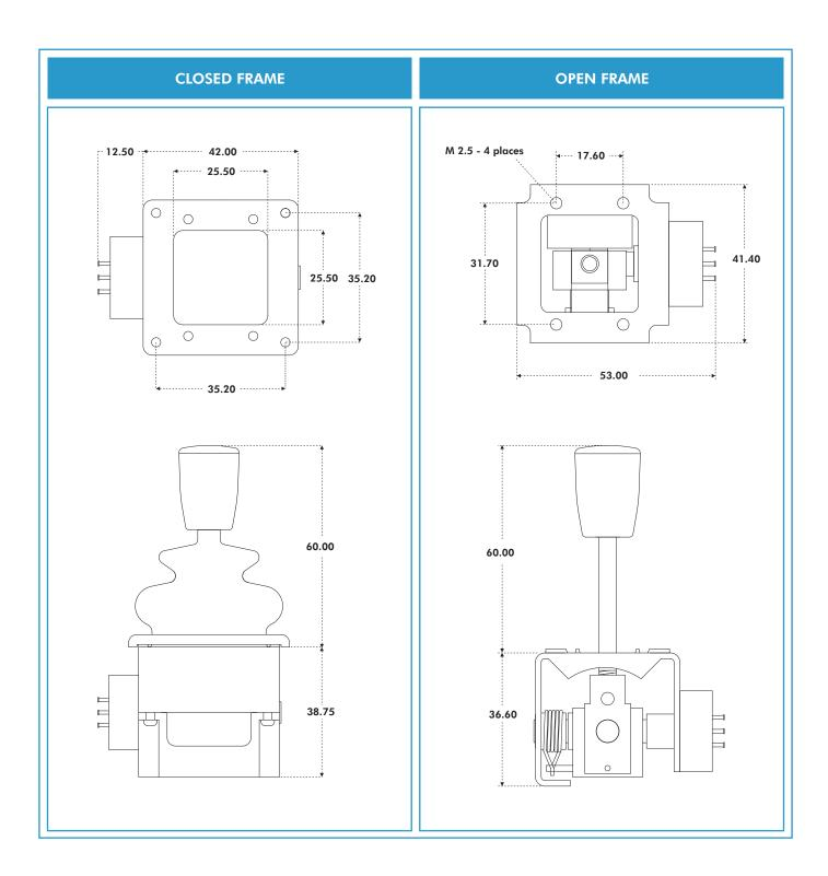
Note: The dimensions shown are for a generic two axes 4000 Series open frame with the E type handle, and a generic two axes 4000 Series closed frame also with the two axes E type handle.
