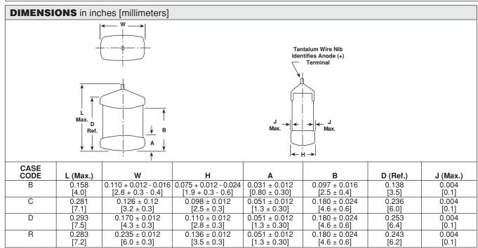
Note: The anode termination (D less B) will be a minimum of 0.012" [0.3mm]
