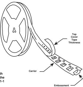
Standard orientation is with the cathode (-) nearest to the sprocket holes per EIA-481-1 and IEC 286-3.
