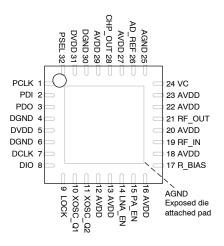
Figure 1. **CC1021** package (top view)
