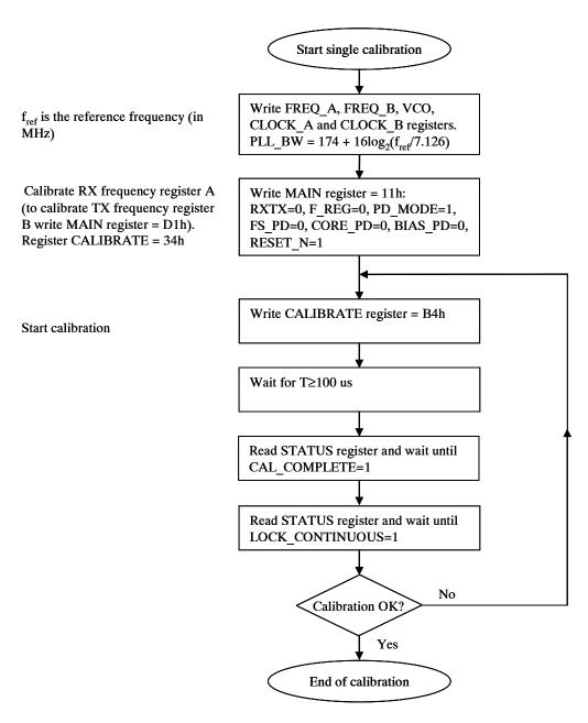
Figure 29. Single calibration algorithm for RX and TX
