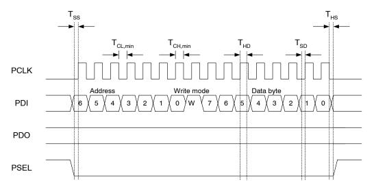
Figure 7. Configuration registers write operation
