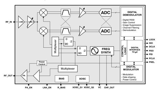
Figure 2. **CC1021** simplified block diagram
