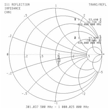
Figure 26. Typical LNA input impedance, 200 ñ 1000 MHz
