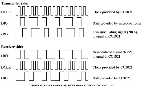
Figure 9. Synchronous NRZ mode (SEP\_DI\_DO = 0)
