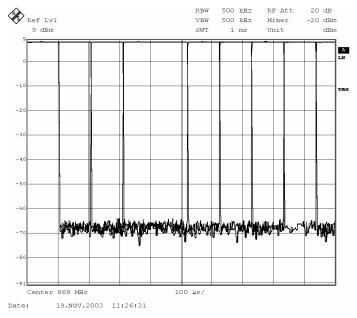
Figure 32. OOK eye diagram. 9.6 kBaud.
