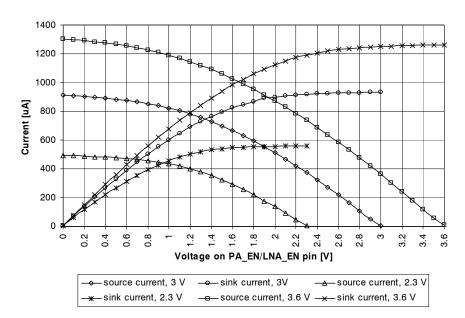
Figure 35. PA\_EN and LNA\_EN pin drive
