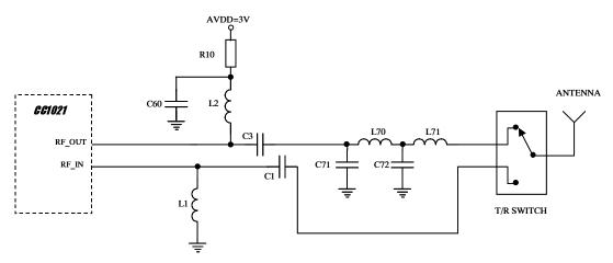
Figure 25. Input/output matching network
