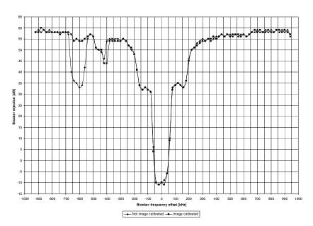
Figure 16. Typical blocker rejection. Carrier frequency set to 434.3072 MHz (102.4 kHz channel filter bandwidth, 19.2 kBaud)
