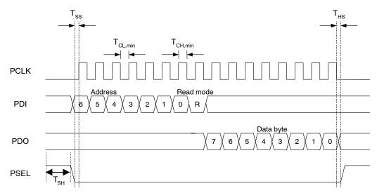
Figure 8. Configuration registers read operation
