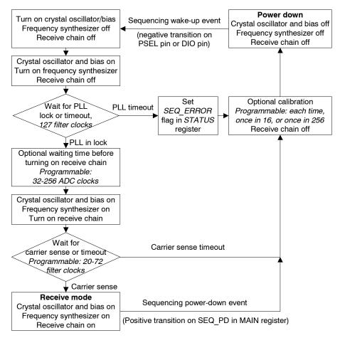
Figure 21. Automatic power-up sequencing flow chart
