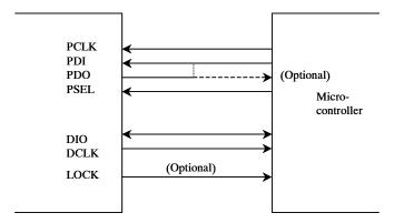
Figure 6. Microcontroller interface
