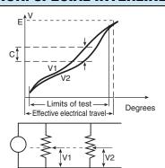
It is the maximum deviation between the actual voltage outputs of 2 or more pot modules in the same assembly. It is expressed as a percentage of the total applied voltage, or in dB attenuation.
