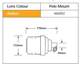
7.24V 120 Gamma Star 60cd (amber) 75/min single flash 356mA 280mA IP55 0.325kg Durastrobe 50cd (amber) IP65 0.325kg 75/min single flash 340mA 186mA
