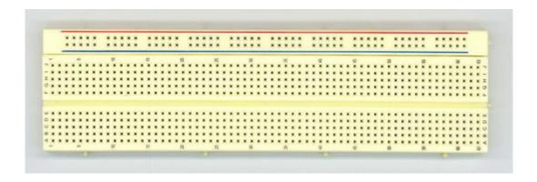
Material: high class POM plastic steel, Dimension: 166 x 45 x 11mm, Distribution strips: 1, Distribution holes: 100, Terminal strips: 1, Terminal holes: 630, Aluminum plate thick: 0.4, With paper box or skin packing
