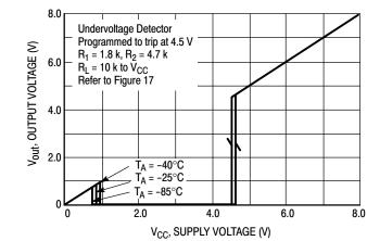
Figure 5. Output Voltage versus Supply Voltage
