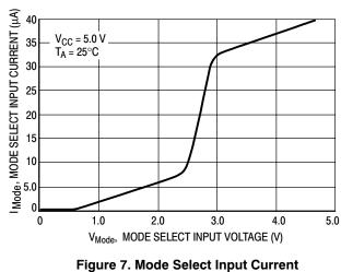
igure 7. Mode Select Input Curren versus Input Voltage
