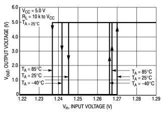
Figure 2. Comparator Input Threshold Voltage
