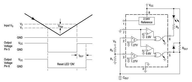
The above figure shows the MC34161 configured as a microprocessor reset with a time delay. Channel 2 monitors input voltage V<sub>S</sub> while channel 1 performs the time delay function. As the input voltage decreases towards ground, the output of channel 2 quickly discharges C<sub>DLY</sub> when V<sub>S</sub> falls below V<sub>1</sub>. As the input voltage increases from ground, the output of channel 2 allows R<sub>DLY</sub> to charge C<sub>DLY</sub> when V<sub>S</sub> exceeds V<sub>2</sub>.
