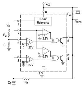
The above figure shows the MC34161 configured as an overvoltage detector with an audio alarm. Channel 1 monitors input voltage V<sub>S</sub> while channel 2 is connected as a simple RC oscillator. As the input voltage increases from ground, the output of channel 1 allows the oscillator to turn 'ON' when Vs exceeds V<sub>2</sub>.
