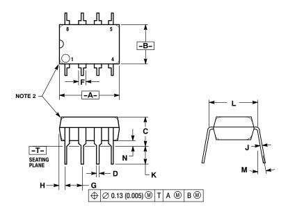
NOTES: 1. DIMENSION L TO CENTER OF LEAD WHEN FORMED PARALLEL. 2. PACKAGE CONTOUR OPTIONAL (ROUND OR SQUARE CORNERS). 3. DIMENSIONING AND TOLERANCING PER ANSI Y14.5M, 1982.
