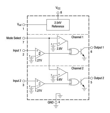
Figure 14. MC34161 Representative Block Diagram
