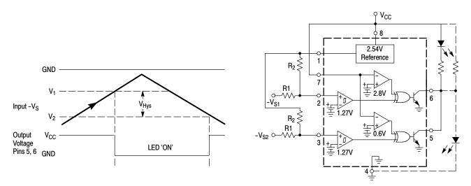
The above figure shows the MC34161 configured as a dual negative undervoltage detector. As the input voltage decreases towards ground, the LED will turn 'ON' when -V<sub>S1</sub> or -V<sub>S2</sub> falls below V<sub>1</sub>. With the dashed line output connection, the circuit becomes a dual negative overvoltage detector. As the input voltage increases from ground, the LED will turn 'ON' when  $-V_{S1} \mbox{ or } -V_{S2} \mbox{ exceeds } V_2.$
