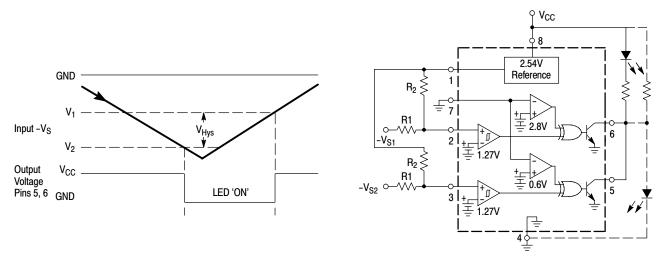
The above figure shows the MC34161 configured as a dual negative overvoltage detector. As the input voltage increases from ground, the LED will turn 'ON' when  $-V_{S1}$  or  $-V_{S2}$  exceeds  $V_2$ . With the dashed line output connection, the circuit becomes a dual negative undervoltage detector. As the input voltage decreases from the peak towards ground, the LED will turn 'ON' when  $-V_{S1}$  or  $-V_{S2}$  falls below  $V_1$ .
