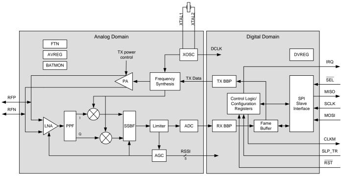
Figure 3-1. Block Diagram of the AT86RF230
