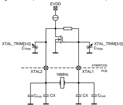
Figure 8-5. Simplified XOSC Schematic with External Components
