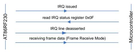
Figure 6-5. Frame Receive Transactions Between AT86RF230 and Microcontroller
