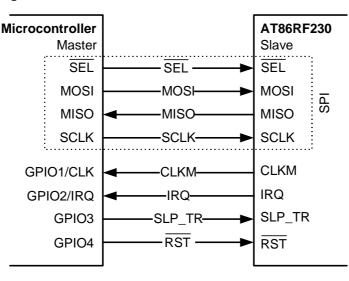
Figure 6-1. Microcontroller to AT86RF230 Interface
