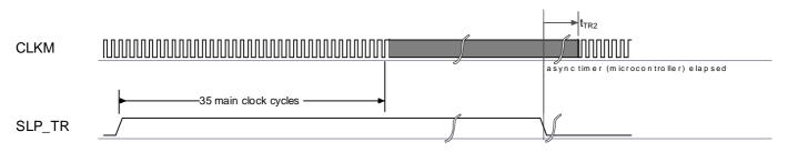
Secondly, if an incoming frame is expected and no other application is running on the microcontroller, the microcontroller can be powered down without missing incoming frames. This scenario is shown in **Figure 6-14**. In RX\_ON state, the CLKM pin is switched off after 35 clock cycles when setting the pin SLP\_TR = H. The radio transceiver state changes to RX\_ON\_NOCLK. The start of a frame reception is indicated by an RX\_START interrupt and the clock is switched on again.
