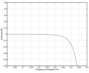
Figure 25. Double-Speed (slow) Passband Detail
