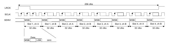
Figure 12. TDM Mode Timing
