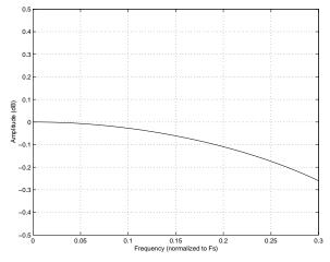
Figure 26. Quad-Speed (fast) Passband Detail
