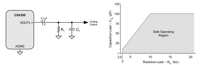
Figure 1. Equivalent Output Load
