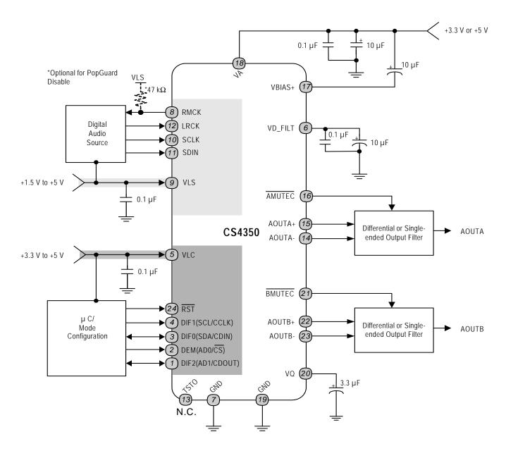
Figure 7. Typical Connection Diagram
