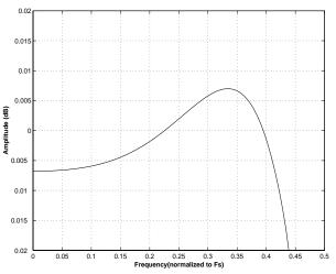
Figure 23. Single-Speed (slow) Passband Detail
