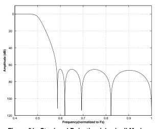
Figure 21. Stopband Rejection (slow), all Modes
