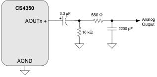
Figure 15. Passive Single-Ended Output Filter
