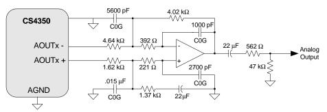
Figure 14. Differential to Single-Ended Output Filter
