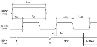
Figure 4. Serial Port Timing, TDM Mode
