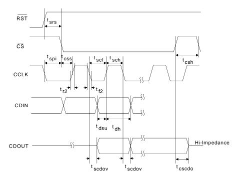
Figure 6. Control Port Timing - SPI Mode
