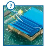
Inspect the installation. Double check to make sure the Heat Sink is securley attached.
