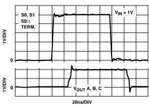
FIGURE 22. CHANNEL TO CHANNEL TRANSIENT RESPONSE  $V_{\text{IN}} = 1V$
