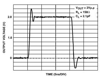
FIGURE 18. LARGE SIGNAL TRANSIENT RESPONSE;  $\mathbf{R_L} = \mathbf{150}\Omega$
