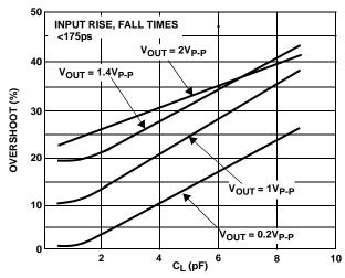
FIGURE 20. PULSE OVERSHOOT vs  $\text{V}_{\mbox{OUT}},\,\text{C}_{\mbox{L}};\,\text{R}_{\mbox{L}}$  = 150 $\Omega$
