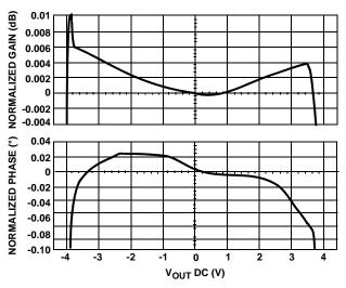
FIGURE 14. DIFFERENTIAL GAIN AND PHASE;  $V_{OUT} = 0.2 V_{P-P}, \, F_O = 3.58 \text{MHz}, \, R_L = 150 \Omega$
