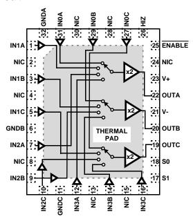
THERMAL PAD INTERNALLY CONNECTED TO V-. PAD MUST BE TIED TO V-
