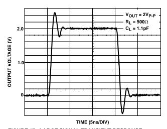
FIGURE 17. LARGE SIGNAL TRANSIENT RESPONSE;  $R_L = 500 \Omega \label{eq:RL}$
