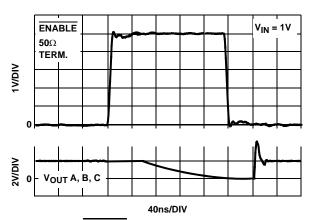
FIGURE 24. ENABLE TRANSIENT RESPONSE VIN = 1V
