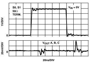
FIGURE 21. CHANNEL TO CHANNEL SWITCHING GLITCH  $V_{\text{IN}} = 0 \text{V}$
