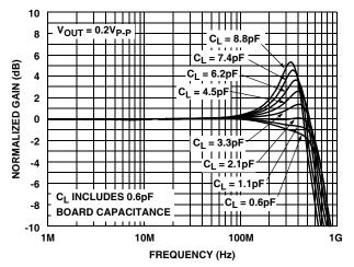
FIGURE 1. SMALL SIGNAL GAIN vs FREQUENCY vs  $C_L$  INTO 500 $\Omega$  LOAD
