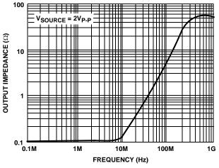
FIGURE 7. Z<sub>OUT</sub> vs FREQUENCY - ENABLED
