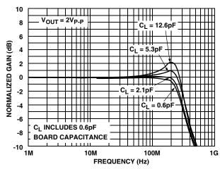
FIGURE 4. LARGE SIGNAL GAIN vs FREQUENCY vs  $C_L$  INTO 150 $\Omega$  LOAD
