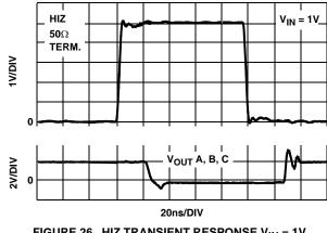
FIGURE 26. HIZ TRANSIENT RESPONSE  $V_{IN} = 1V$
