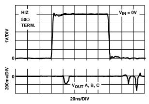
FIGURE 25. HIZ SWITCHING GLITCH  $V_{IN} = 0V$
