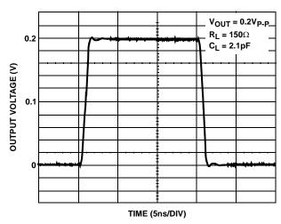
FIGURE 16. SMALL SIGNAL TRANSIENT RESPONSE;  $\mathbf{R_L} = \mathbf{150}\Omega$
