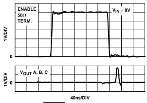
FIGURE 23. ENABLE SWITCHING GLITCH VIN = 0V
