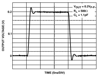
FIGURE 15. SMALL SIGNAL TRANSIENT RESPONSE;  $R_L = 500 \Omega \label{eq:RL}$
