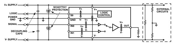
FIGURE 30. SCHOTTKY PROTECTION CIRCUIT
