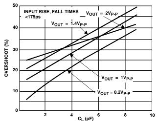
FIGURE 19. PULSE OVERSHOOT vs V $_{OUT}$ ,  $C_L$ ;  $R_L$  = 500 $\Omega$
