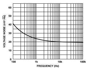
FIGURE 12. INPUT NOISE vs FREQUENCY
