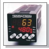
The TE48 is a panel mounting or plugin programmable timer, packaged in a 1/16th DIN IP65 rated housing and is an extremely versatile product offering 11 operating modes applied to two timed output relay contacts. When only one of the timers is being used, the other output acts as an instantaneous set of changeover contacts. A single model provides timing from 0.1 seconds to 100 hours.
