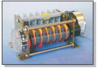
The 5000 series electromechanical cam timers can be supplied with either 2, 4 or 6 cams. The standard models are supplied with 2 screw adjustable cams at each micro switch position. Cycle times between 3 seconds and 24 hours can be achieved using the standard motor and gearbox combination.
