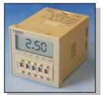
The LE3S timer has 10 operating modes and 10 time ranges, all selectable from the front panel. The LCD display shows the state of the output and a bar graph of the timing cycle as well as the 3 digit process time display. The single model is powered from 100 to 240Vac or 24 to 240Vdc. The LE3S is housed in a compact 1/16 DIN 48 x 48 mm case.
