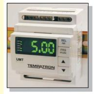
The UMT 500 timer is a programmable digital timer with 5 relay outputs, each of which has 5 selectable operating modes and an external start/reset function. Each output can either be programmed in timed or instantaneous mode making the UMT500 a particularly flexible unit for in-panel machine control applications that do not warrant the cost or complexity of an industrial plc.
