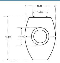
A multi functional handle with two momentary IS Series switches one on top and one on the front.
