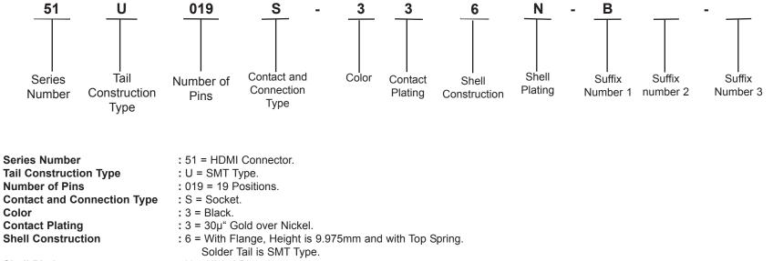
Shell Plating: N = Nickel Plated.Suffix Number 1: B = Without Freeport Logo.Suffix Number 2: None = PVC Tray Package.Suffix Number 3: None = Shell Material is Phosphor Bronze.
