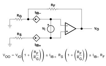
Figure 29. Output Offset Voltage Model
