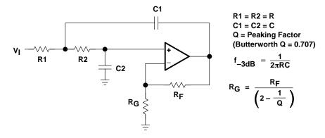
Figure 32. 2-Pole Low-Pass Sallen-Key Filter
