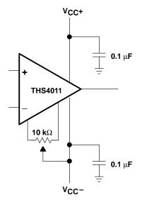
Figure 28. Offset Nulling Schematic
