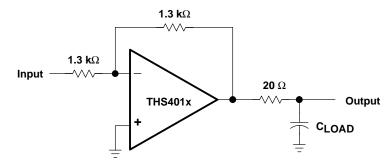
Figure 27. Driving a Capacitive Load
