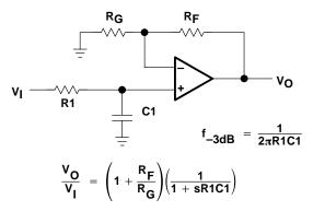
Figure 31. Single-Pole Low-Pass Filter
