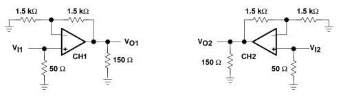
Figure 3. THS4012 Crosstalk Test Circuit
