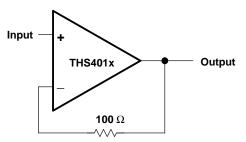
Figure 30. Noninverting, Unity Gain Schematic
