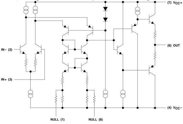
Figure 24. THS4011 Simplified Schematic
