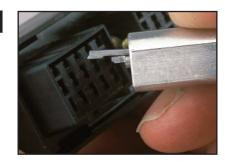
Hold connector with cavity letter and number identification in the upright position. Terminal removal tool is to be inserted in the front of the cavity, opposite to the wires.
