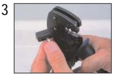
Insert an individual terminal into the proper window as directed by wire gauge indicators on the tool.
