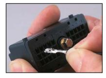
Grasp connector with cavity letter and number identification in the upright position.
