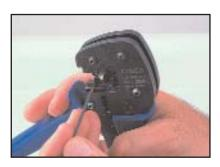
Pre-strip wire to required specification shown below (4.85 mm / 0.191 inches). Insert the pre-stripped wire into the terminal located in the hand tool.
