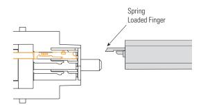
The tool is designed so that the longer spring loaded finger lifts the latch out of the terminal locking window. The shorter finger is stationary and will push out the terminal once the latch is lifted.
