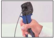
With the terminal and wire set in the proper position, (see above) hold the wire stationary and squeeze the tool together. Complete the crimp by squeezing the tool until the ratchet releases. Remove the terminated wire from the tool.
