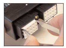
Push Tweezer in and squeeze to depress the locking tabs. Hold squeeze and pull secondary lock out of the connector.
