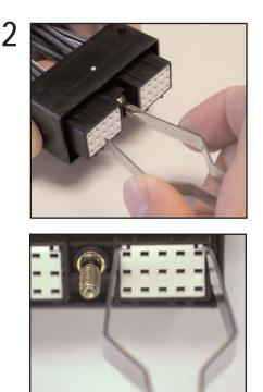
Insert tips of the tool besides the secondary lock locking tabs.
