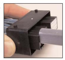
Push removal tool straight in so it bottoms against the connector.
