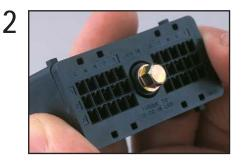
Secure the insulator in place by holding it in one hand. Make sure that Cavity Identification letters are in the upright position. (Shown below).
