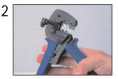
With hand tool in ready position, (open handle) open the terminal receptacle.
