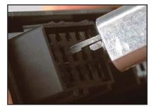
Locate wire to be extracted and its cavity in the front of the connector. Insert removal tool straight in with the spring loaded finger in the upright position.
