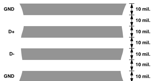
Figure 17. Arrangement of Signal Tracks
