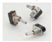
The 110-Series is a compactly designed, versatile metal construction toggle switch. Features include single or double pole options, maintained or momentary construction with termination choices including solder lug end or bottom, wire leads and .250 tab terminals. The quick make/quick break contact mechanism makes the switch suitable for high voltage (125-250 volt) applications. This switch is popular within the Small Appliance, Floor Maintenance, and most low current AC/DC market segments.
