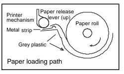
mechanism grips the paper and feeds it through. There is an optical sensor which "sees" the paper and will drive the motor for a predetermined time. If the paper fails to grip and advance the paper, withdraw the paper and try again. When it reappears above the rubber, press the paper feed button, and allow enough to feed through for good alignment, thread the paper through the exit slot and close the lid.
