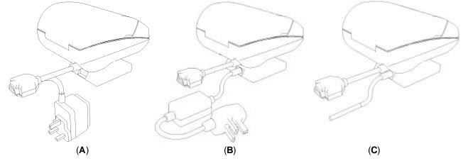
All three options are housed in the same type of replaceable pack, which clips into the underside of the printer and can be changed in a few seconds by the user. In each case, the primary power for the printer comes from this replaceable pack.
