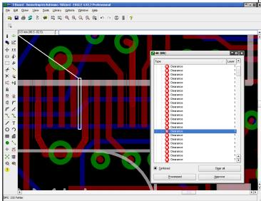
To rule out the possibility of errors caused by the manual work, EAGLE carries out a Design Rule Check (DRC). This will check whether, for example, there are shortcircuits on the board, or whether different potentials are too close to one another.
