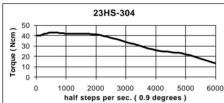
Coils in parallel, 2.0 amps per phase
