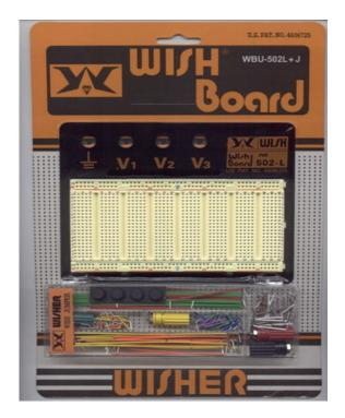
Material: high class POM plastic steel, Dimension: 125 x 160 x 31mm Distribution strips: 2, Distribution holes: 170, Terminal strips: 1, Terminal holes: 800, Aluminum plate thick: 1.5, Knob posts: 4, Foot pads: 4 with jumper wire With skin packing.
