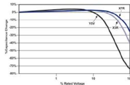
**Figure 8 - Typical Variation of Capacitance with Applied DC Voltage**
