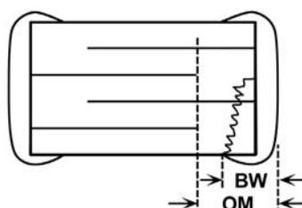
The open-mode dimension (OM) exceeds the termination bandwidth dimensions: OM > BW
