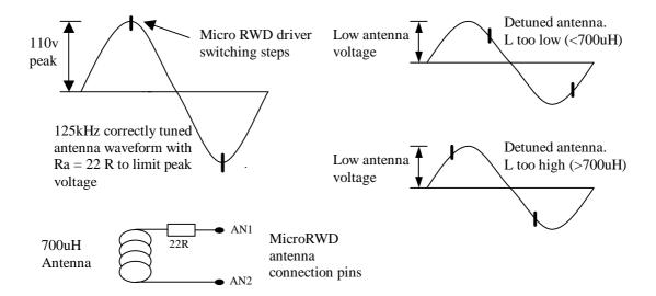
6) For optimum performance the antenna Q should not exceed 20 and to achieve reliable tuning at 125kHz the antenna inductance should be around 700uH. Higher Q and inductance values will still function but with a reduced range and performance.
